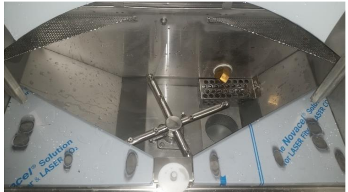
Wash cabinet and wash arm
