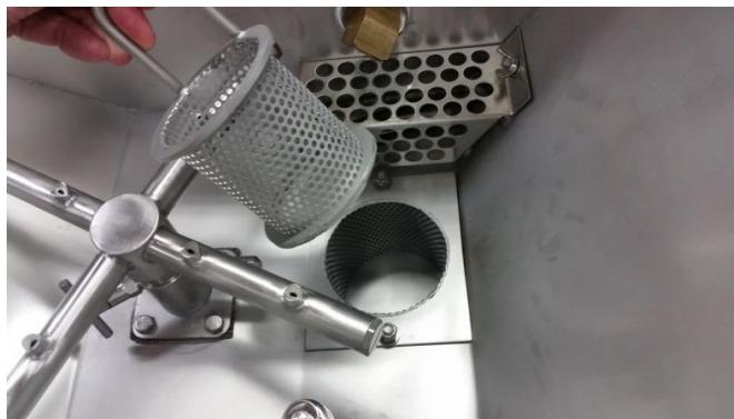
Pump filter (085-6218), Placement of the pump filter into the drain sump
