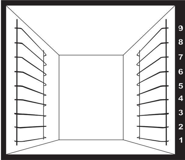
1. **POSITION** The best arrangement for broiling, baking cookies and for other baked goods under 2-1/2" (65mm) in height. This arrangement can also be used as the maximum capacity for reconstituting frozen entrées.
