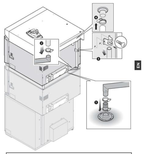
A second oven must be connected using the extension included in the stacking kit
