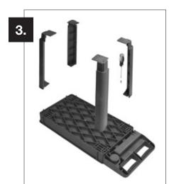
Use 3 screws to secure each leg to frame
