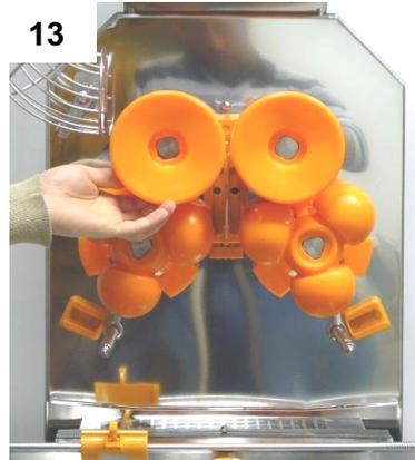
12. Remove the peel ejectors left and right (Pic 12).
