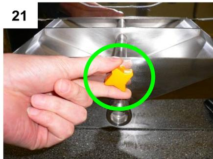
21. Unscrew the fruit sieve support nut and remove the sieve support (Pic 20).
