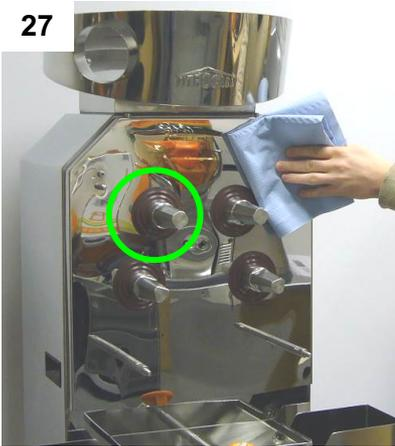
27. Wipe down the housing with warm, clean water and a soft cloth (Pic 27). Dry thoroughly before reassembling the machine. Be sure to wipe down the stainless-steel posts to remove any juice residue.
