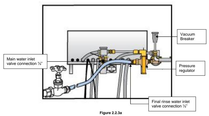
To set the final rinse pressure, the final rinse must be running. Turn the adjustment screw clockwise to increase final rinse pressure; and counter-clockwise to decrease the pressure set the final rinse pressure to 20-psi ±5 psi. (Set to 22 - 23 psi for optimum running pressure)
