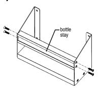
Step 4 - Affix bottle labels (not included) onto top of stay, as needed. Snap clear molding onto bottle stay.
