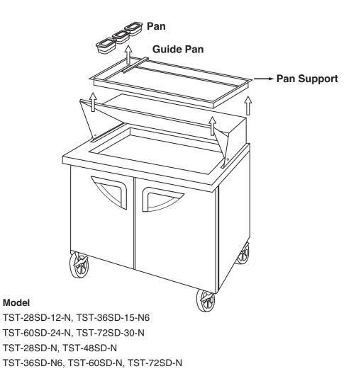
Remove the Guide Pans and Pans. Then pull out the Pan Supporter. Clean the pan supporter and reinstall in place.
