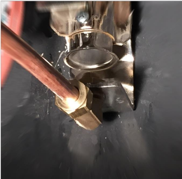
Fig 7.2 Nozzle-holder curve and damper sleeve
