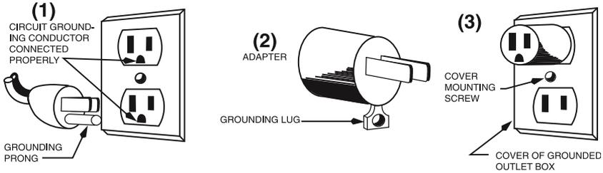
If a grounding-type outlet is not available, an adapter, shown in Figure 2, may be obtained so that a 2-slot wall outlet can be used with a 3-prong plug. As shown in Figure 3, the adapter must be grounded by attaching its grounding lug under the screw of the outlet cover plate.
