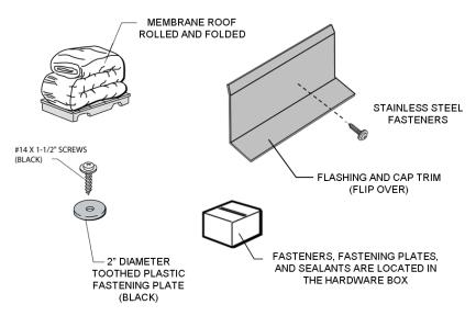
Check the roof of the walk-in unit and remove any foreign matter. Seal all protruding rough edges and screw heads, rivets, etc. with tape or sealant. This will prevent any chance of penetrating or wearing a hole in the membrane roof cap.
