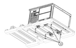
**NOTE:** Traulsen does not recommend laying the unit on its front, side or back. If you must, please allow the unit to remain in an upright position for 24 hours before plugging it in so that the compressor oils and refrigerant may settle.
