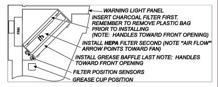
Remove the protective plastic bag from charcoal filter before installing.
