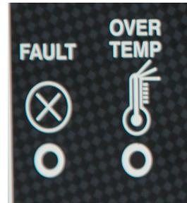
**FAULT - (Gas Only)** When this error is lit an ignition failure of the appliance has occurred. following the following steps:
