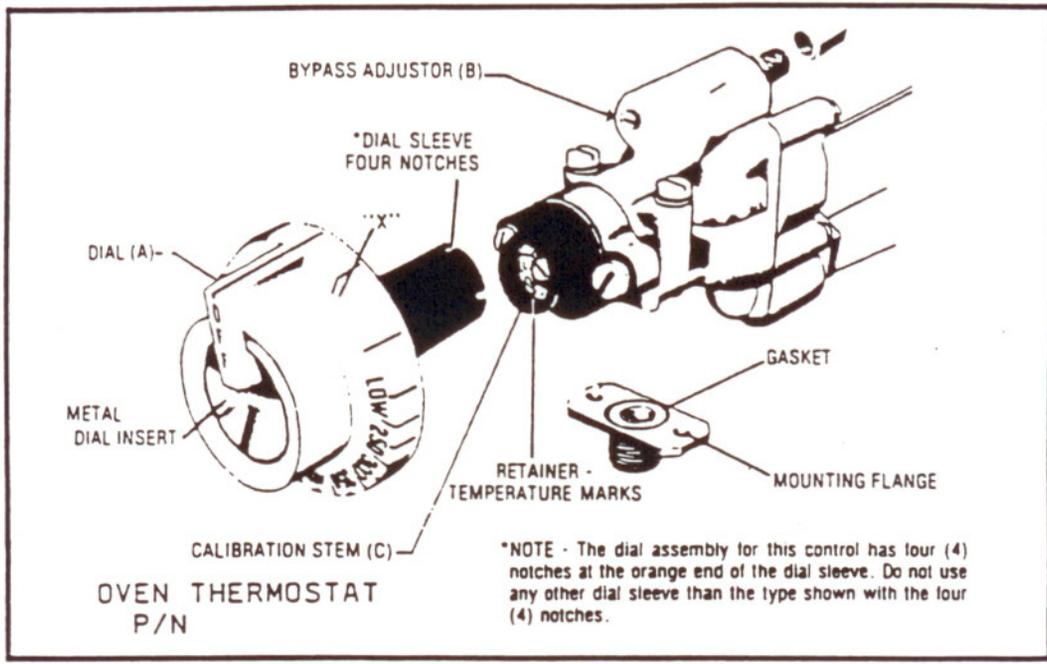
**THE BYPASS MUST BE SET CAREFULLY AND ACCURATELY AS FOLLOWS:**
