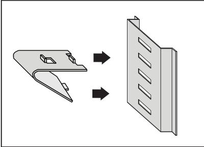
1. Attach the shelf clips onto the pilasters by inserting its top hook into a pilaster notch followed by the bottom hook. Do not use pliers or other crimping tools to modify the shape of the shelf clips. This will result in shelf mounting instability.
