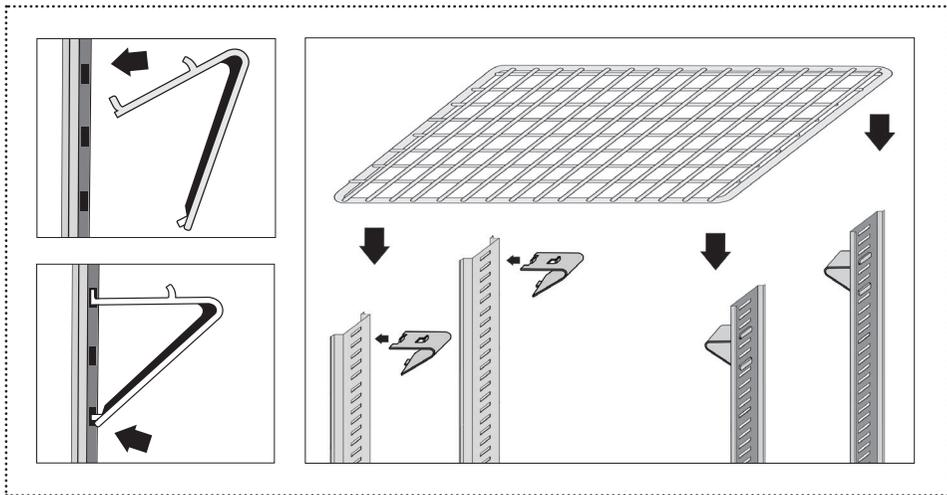
2. Place shelves on the shelf clips making sure all corners are mounted securely and evenly with identical distance from the unit's floor and up. Always lay the back of each shelf down on the rear clips before the front.
