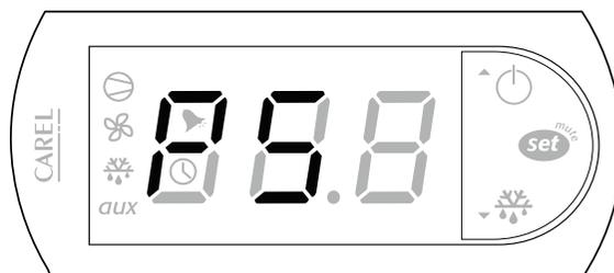
This means the Temperature Set button **set** was held down longer than 3 seconds. To exit this mode and restart, press Temperature Set Button **set**
